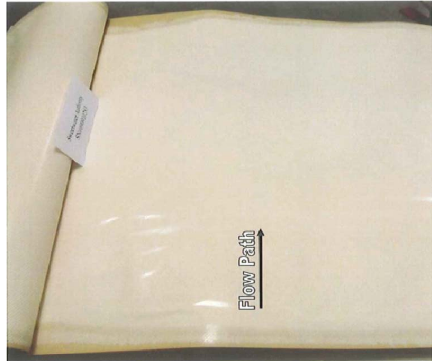
Image of membrane surface from feed end
