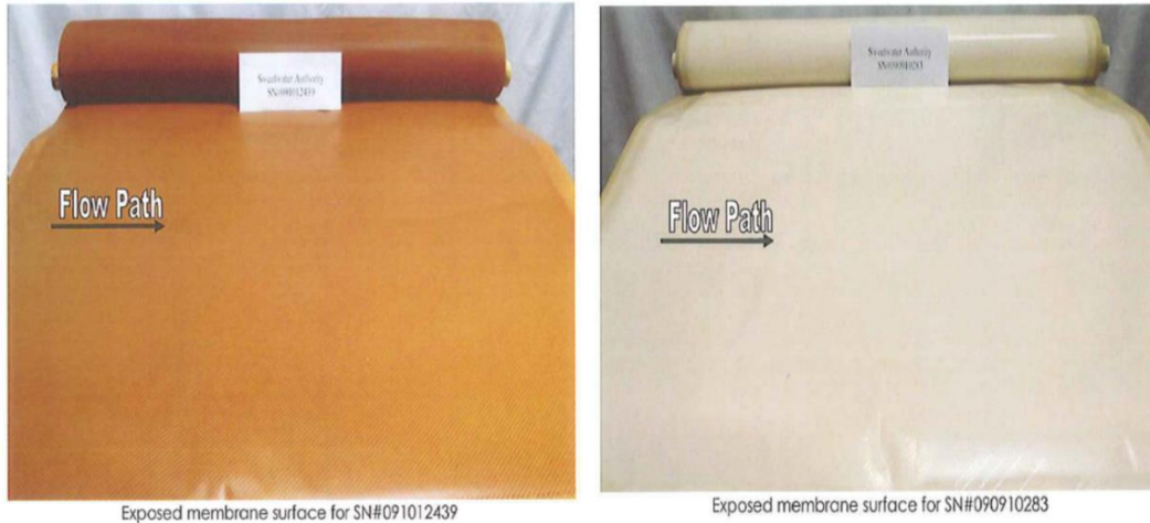
Figure 7: Comparison of Stage 1 and Stage 2 Element Membrane Surfaces
